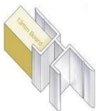
Butt joint / Shadow Gap – GA PTE13SG
