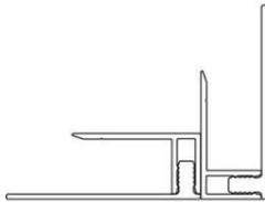
**Internal Corner** (GA IN78) *optional*. C/w pre-drilled holes for 3.5mm Ø screws.
